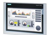
SIMATIC HMI TP1200 Comfort, Comfort Panel, touch operation, 12" widescreen TFT display, 16 million colors, PROFINET interface, MPI/PROFIBUS DP interface, 12 MB configuration memory, Windows CE 6.0, configurable from WinCC Comfort V11
